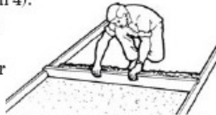
(Diagram 4 - Screeding the sand)
