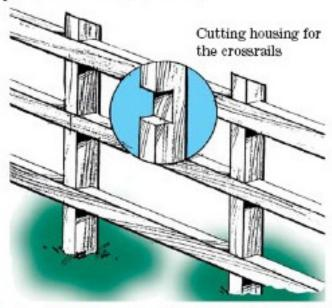
Fix the rails to the posts with two 75 x 3.75mm galvanised bullet head nails. Joins in the rails should be butted together in the centre of the post notch. Stagger the joins in the rails over different posts.
