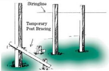
Place the posts central in the holes and attach two braces as shown. Plumb the posts with a spirit level and fasten the braces securely. If the soil is sandy then additional braces below the ground are required, as shown.
