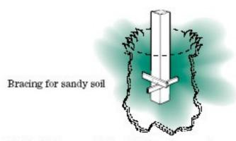
Fill the holes completely with Premix concrete, or make up a cement-soil mix (6 parts soil to 1 part cement) and consolidate by hard ramming with a crow bar. Check the posts with a spirit level and adjust to plumb if necessary. The top of the footings should be sloped away from the posts to drain away water. The remainder of the posts can be installed in the same way, using a string line to ensure that they all are in a straight line. Allow a few days for the cement to cure before proceeding.
